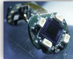
*Pillcam CMOS Image Sensor*
