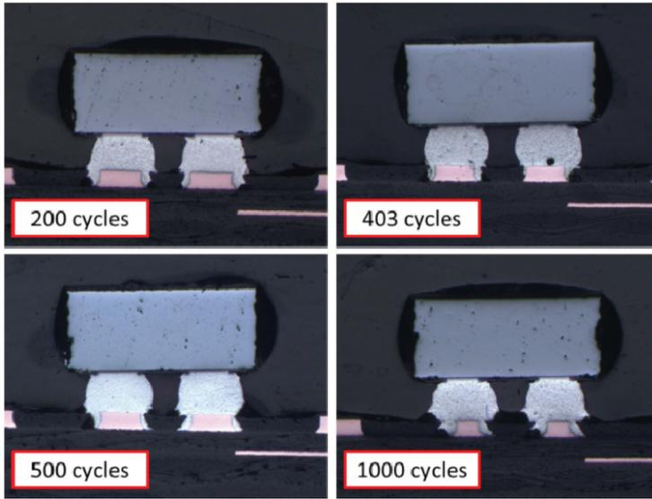
Figure 9: Cross sections of FC (ID #5) after thermal cycling.
