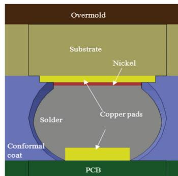
Figure 13. FE model structure with Thick conformal coating.
