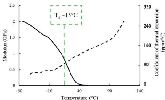
Figure 1. DMA and TMA results of acrylic coating.
