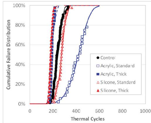
Figure 4: BGA reliability: SAC305 solder, -55 to +125°C thermal cycle profile.
