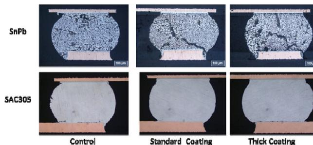
Figure 7: Cross sections of solder joints with silicone conformal coating.
