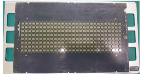
Fig. 12(b). Mesh type carrier boat is needed for thin coreless substrates.
