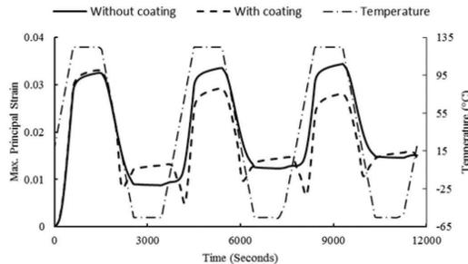
Figure 15. Maximum principal strain over time and temperature with and without conformal coating for SAC305 corner solder joint under Temperature Profile 1.
