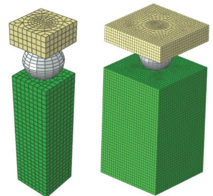
Figure 11. Local model 'plugs': (a) solder joint with coarse mesh; (b) solder joint with fine mesh.
