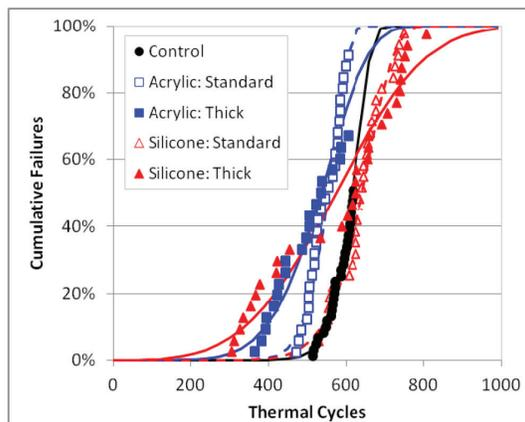
Figure 3: BGA reliability: SnPb solder, -55 to +125°C thermal cycle profile.
