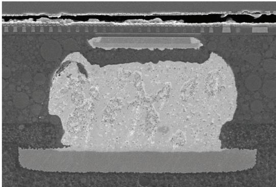
Fig. 11. Bump IMC crack and die crack due to substrate warpage during reflow.
