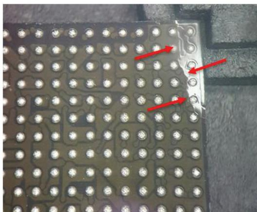
Fig. 15. Substrate crack during assembly/test.
