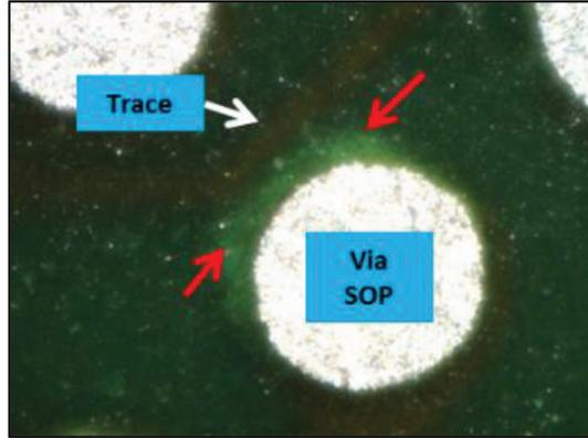
Fig. 4. Optical image of via solder-on-pad (SOP) with solder extrusion.
