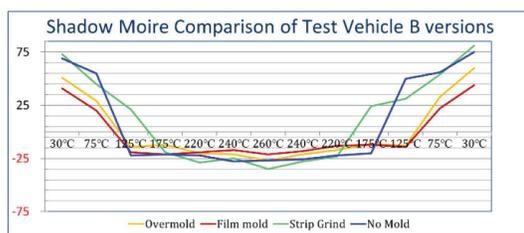
Fig. 9. Shadow Moiré of various lidless package process techniques in comparison with overmolded package.
