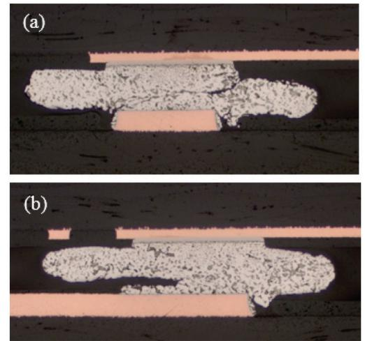
Figure 10. Sn63Pb37 corner BGA with thick acrylic coating survived 1600 cycles: (a) corner joint; (b) joint in middle row.
