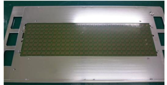
Fig. 12(a). Normal substrate carrier boat which is used for thicker substrates.
