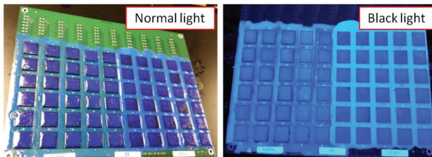
Figure 2: Conformally coated BGA test board (left side has 'Standard' coating; right side has 'Thick' coating).
