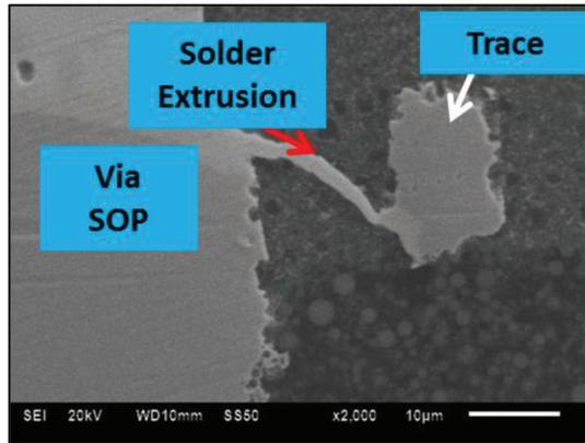
Fig. 5. Cross-section SEM image of solder extrusion and solder bridging between via solder-on-pad (SOP) and adjoining trace.
