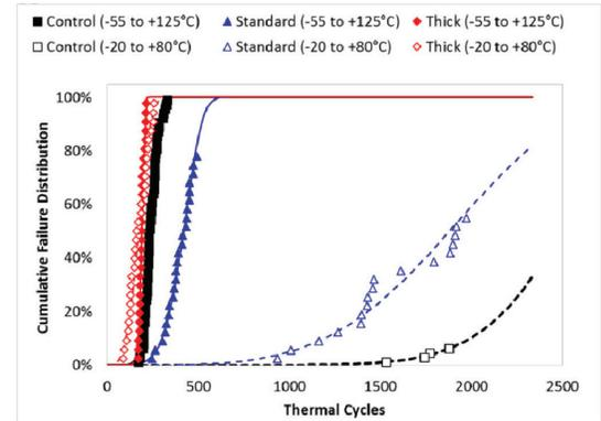
Figure 4. Cumulative failure distribution for the SAC305 samples with Standard and Thick acrylic coating. Solid lines/ symbols correspond to -55 to +125°C testing; dashed lines/open symbols correspond to -20 to +80°C testing.
