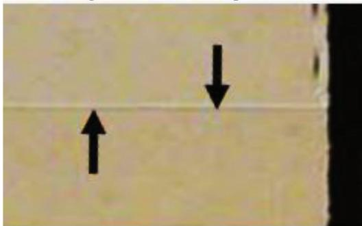
Fig. 13. Backside die crack due to foreign particle on the wafer chuck table during wafer backgrind.
