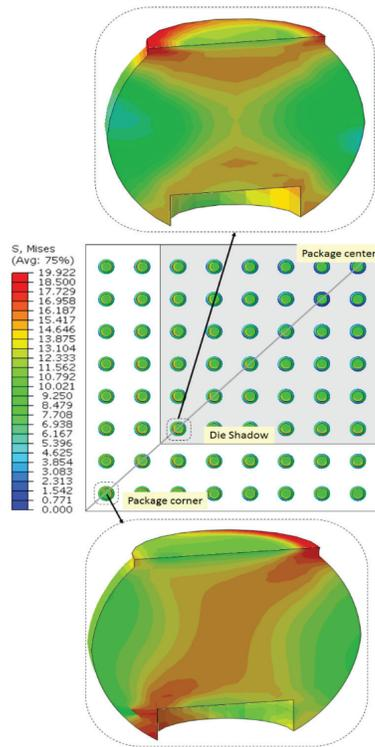
Figure 14. Von Mises stress distribution in SAC305 BGA with Thick conformal coating at 125°C.
