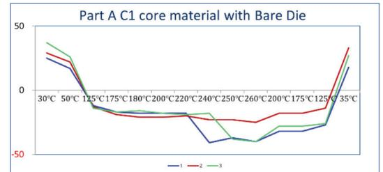
Fig. 6. Shadow Moiré graph of test Vehicle A with V0 substrate with bare die.
