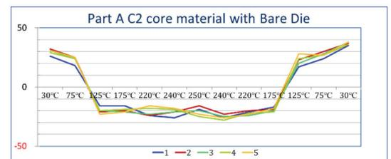
Fig. 7. Shadow Moiré graph of test Vehicle A with V1 substrate with bare die has lower warpage than V0 substrate version.
