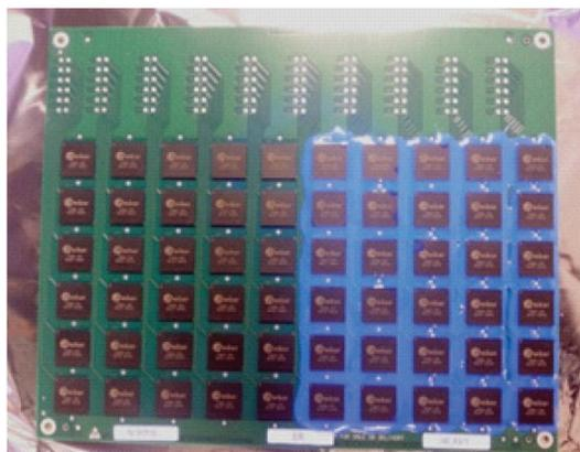
Figure 2. Assembled test vehicle showing two halves of the board with one side applied with Thick conformal coating [7].
