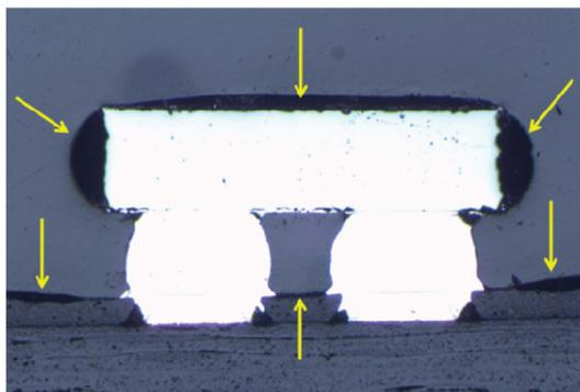
Figure 8: Overexposed image of flip chip cross section (to illustrate conformal coating coverage).
