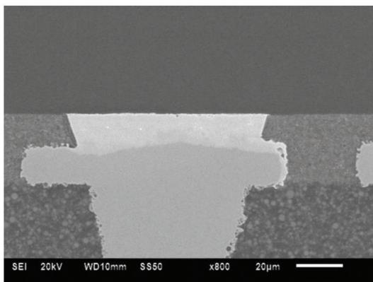
Fig. 8. Cross-section SEM image of critical via in V1 substrate. No solder extrusion was observed.
