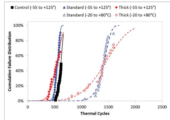
Figure 5. Cumulative failure distribution for the Sn63Pb37 samples with Standard and Thick acrylic coating.
