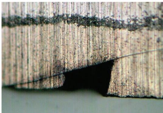
Fig. 14. Backside crack/chipout after wafer saw.
