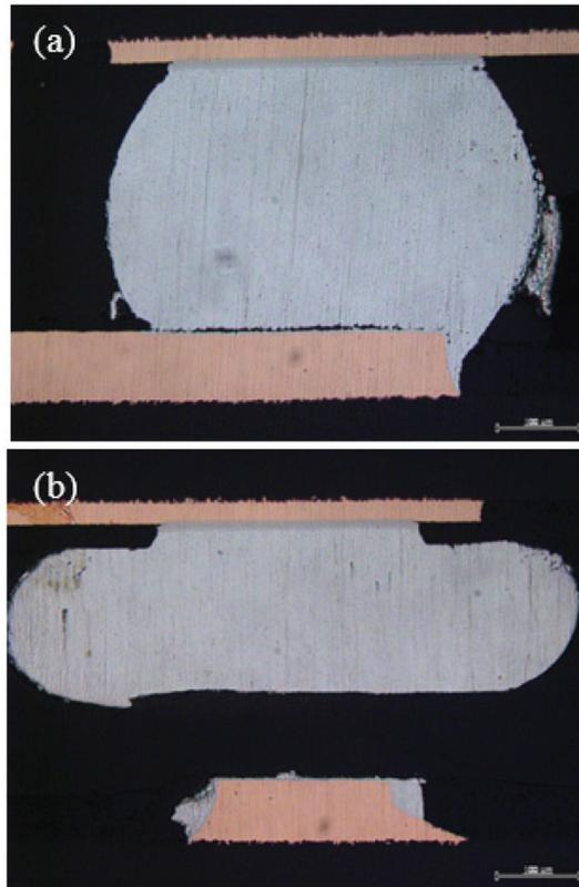
Figure 7. Failure of SAC305 corner BGA with acrylic conformal coating ( $-55$  to  $125^{\circ}\text{C}$ ): (a) Standard; (b) Thick coating.
