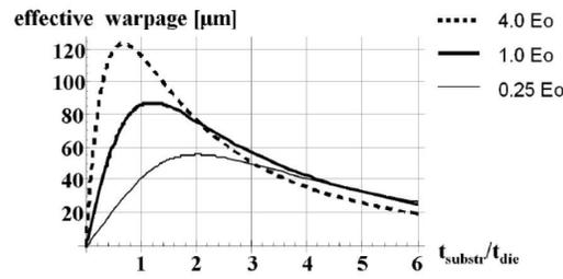
Fig. 2. Effect of substrate to die thickness ratio [4].
