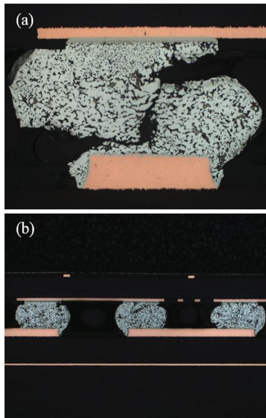
Figure 9. Sn63Pb37 BGA with thick conformal coating failed at 1055 thermal cycles (-20 to 80°C): (a) corner joint; (b) joints in the middle of a row.
