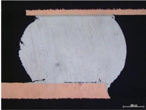
Figure 6. SAC305 corner BGA Control sample (no coating) showing cracking along bottom pad.
