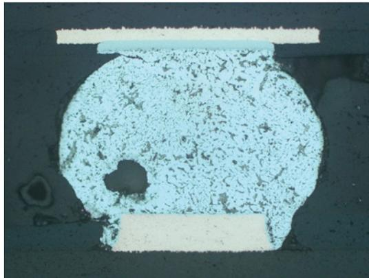
Figure 8. Sn63Pb37 corner BGA with acrylic Standard coating showing cracking in upper left size of solder joint at 1600 cycles.
