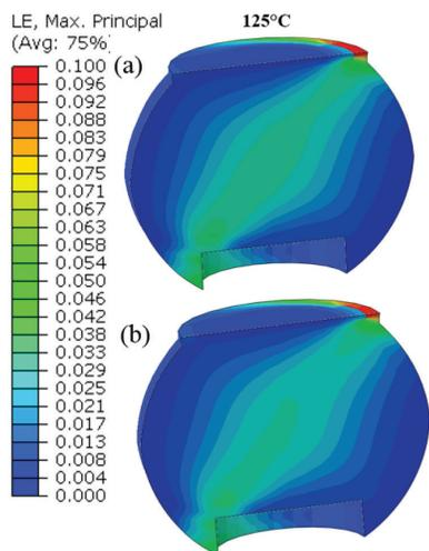
Figure 17. Sn63Pb37 Maximum principal strain at 125°C for the corner BGA: (a) with conformal coating; (b) without conformal coating.
