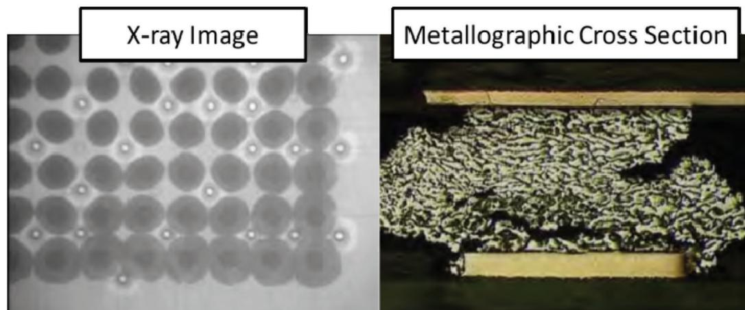
Figure 1: Top and side views of BGA solder joints with improper conformal coating after thermal cycling [1].
