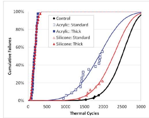
Figure 5: BGA reliability: SAC305 solder, -20 to +80°C thermal cycle profile (courtesy of Maxim Sebrini, DJR Solutions).
