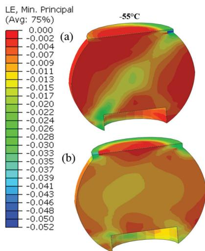
Figure 18. Sn63Pb37 BGA Min. principal strains at -55°C for corner joint: (a) with Thick coating; (b) without Thick coating.
