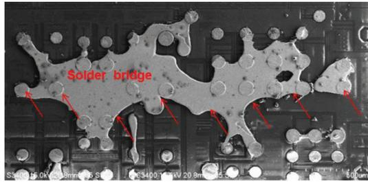
Fig. 10. Solder bump bridging due to molten solder bumps.
