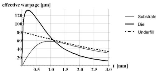
Fig. 1. Effect of thickness of individual layers [4].
