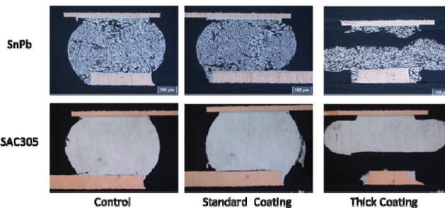
Figure 6: Cross sections of solder joints with acrylic conformal coating.
