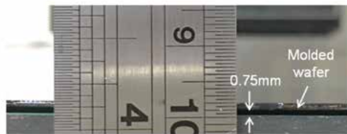
Figure 13. Warpage of molded wafer on glass carrier with CTE of 8 ppm/°C.
