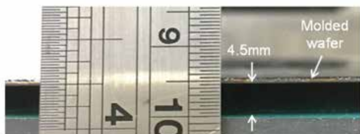
Figure 12. Warpage of molded wafer on glass carrier with CTE of 3 ppm/°C.
