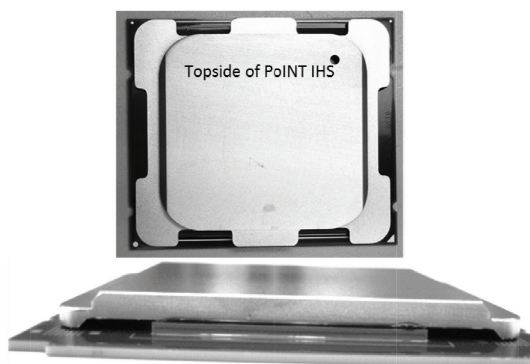
Figure 10. Novel IHS design optimized for PoINT architecture (top and cross-sectional views).
