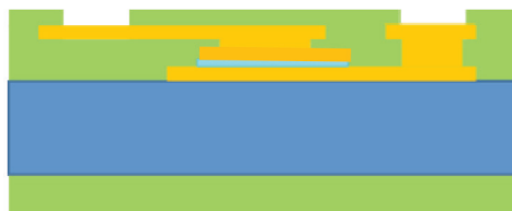
Figure 16. X-section of MIM structure.
