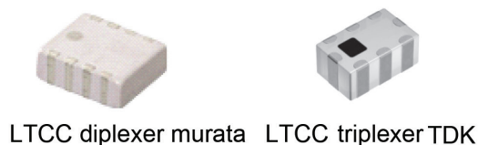
Figure 4. Current multi bands filters using LTCC.
