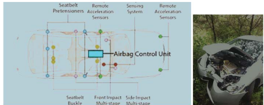
Figure 3: Diagram of (and need for) Safety Sensors including Airbag Control Unit.
