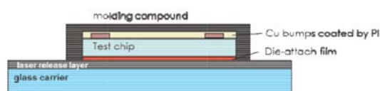
Figure 1. Chip-first and die face-up sample structure.
